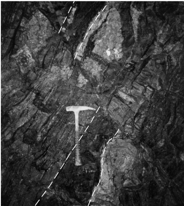
Fig. 4. Amphibolite (outlined) is concordant with the surrounding quartzofeldspathic gneiss (4460 mN, 1821 mE, 887 mRL). Leucosomes range from plagioclase-rich at amphibolite margins (light), to K-feldspar-quartz (dark) within the gneiss. A late fault displaces the amphibolite and gneiss. Hammer for scale.
